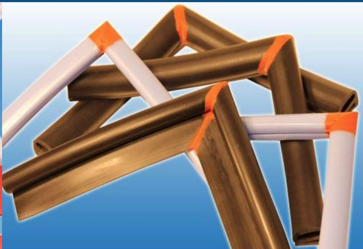
Jehbco Silicones is able to produce a large variety of O'Rings, from Silicone Cords or Silicone Strips. With Cross Sections from 1.0mm up to 40.0mm, and Diameters as large as needed. And Hardness's from 20 shore A up to 80 shore A. They are fabricated with a unique Vulcanizing technique which makes the joints as smooth as molded parts.
