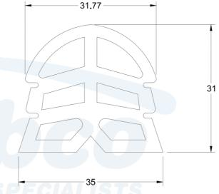
A general tolerance of ±0.2mm is applied for all dimensions in this profile.
