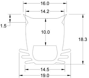
A general tolerance of  $\pm 0.2$ mm is applied for all dimensions in this profile.
